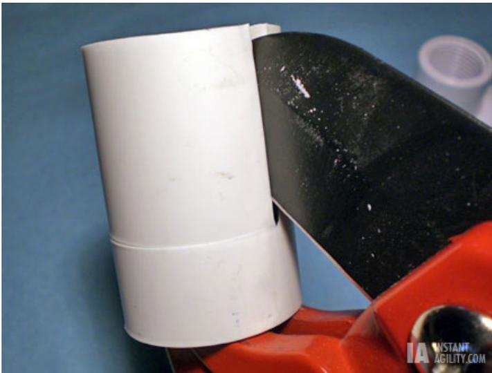
Here the cut is almost complete. You may wish to open the cutter and adjust the pipe so the blade is closer to perpendicular to the pipe for a neater finish.
