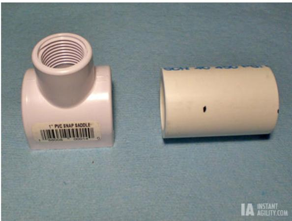
Here are the (uncleaned) pieces you need to make one cup. On the left is the “Snap Saddle” as can be seen from its label, and on the right is a two-inch section of 1” diameter PVC pipe. Make a pen mark  $\frac{3}{4}$ ” from the end of the pipe; this will guide you when making the cut partially through the pipe.
