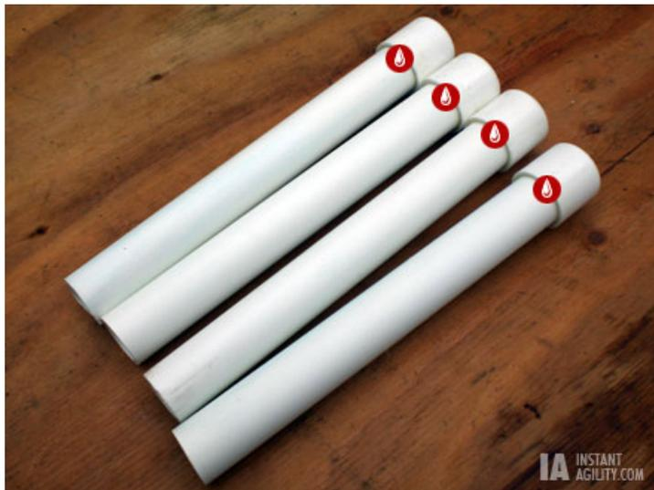
Start by gluing four end caps 1 to the four feet 3.
