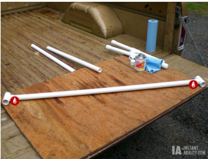
Set aside the feet and glue the two remaining “T” connectors 2 to the 50” cross bar 6. It is important that these two connectors be coplanar. Glue one first and let it set, then glue the other in place ensuring that both connectors are flat on your work surface as shown.
