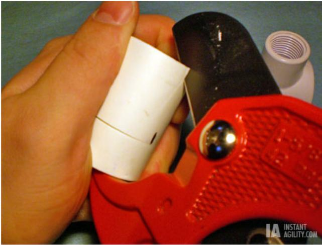
I have made a mark on the pipe to guide me as I place the blade to make the long cut. I eyeballed it by looking at the cutter from above to ensure the mark was under the blade, but you could be more precise by extended the mark out to the end of the pipe.
