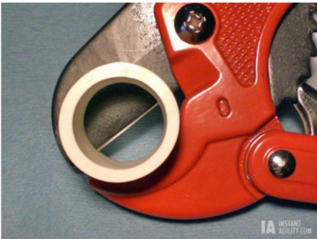
Using the mark you made, cut a little more than halfway through the pipe, as illustrated above. Certain professional organizations have precise measurements for the depth of the cup, but “a bit more than halfway” is fine for casual agility.
